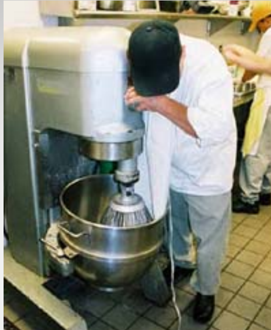
Apron caught in mixer with no guarding
